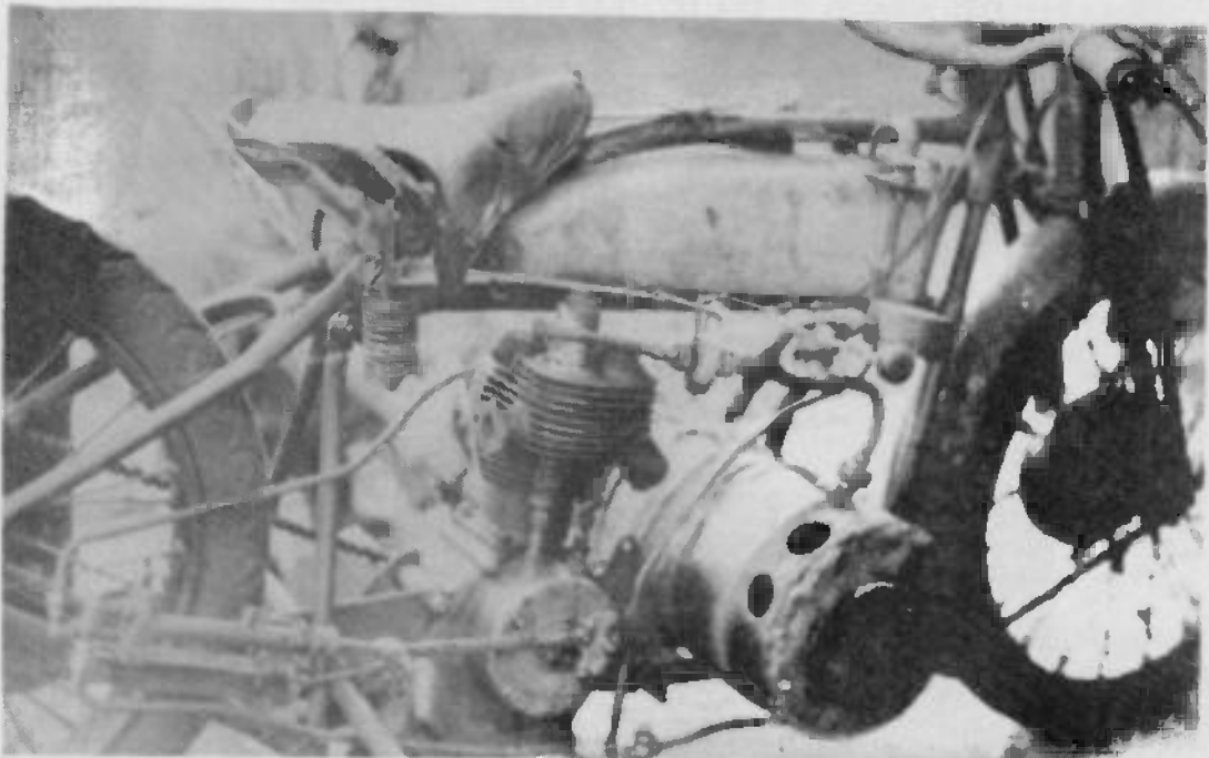
Steam Motorcycle using converted 1924 550 cc. BSA engine Twist grip throttle, Horizontal flash boiler in front. Holes in front casing are for flue gas outlet. Water feed pump driven from timing gear. (Those Stanley pumps really get around.) Owned by Sydney Clement, Pres. Steam Power Unit Development Society of Australia.
