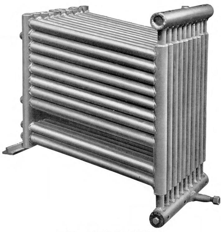
Modern Automobile Water-Tube Boiler
