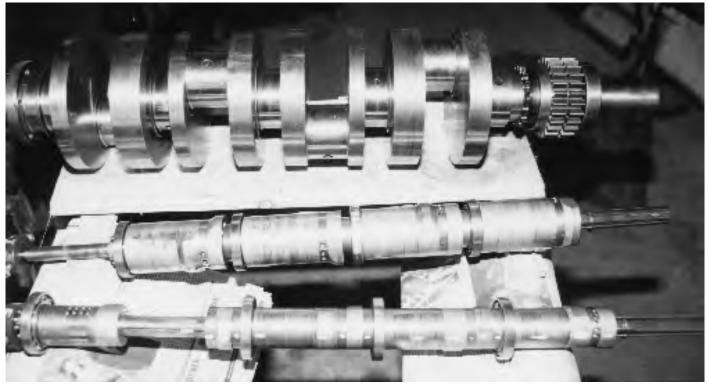
Williams 265 bus engine crankshaft plus two sliding camshafts
