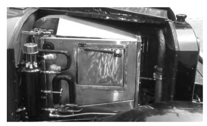
Derr boiler installation in Rolly's 1920 Stanley
