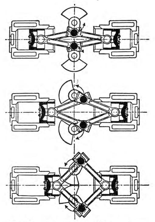
Three phases in the movements of pistons and connecting-rods in the Lanchester engine: (top) the rods nearest to horizontal centre line of the opposed cylinders, lift piston on power stroke; (centre) cranks at TDC for right piston, which is at end of compression stroke; (bottom) the left piston is on BDC and the rods are approaching their widest relative angle
