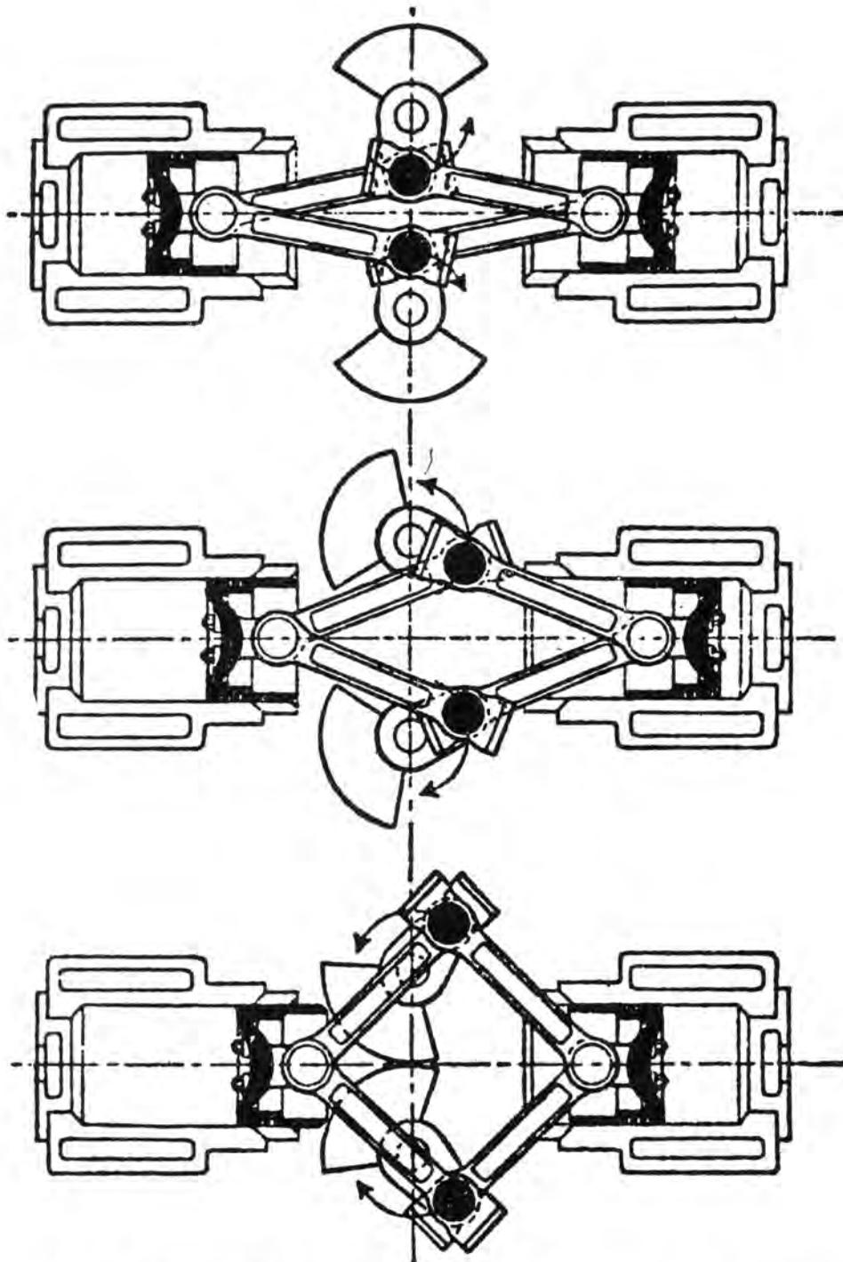
Three phases in the movements of pistons and connecting-rods in the Lanchester engine: (*top*) the rods nearest to horizontal centre line of the opposed cylinders, lift piston on power stroke; (*centre*) cranks at TDC for right piston, which is at end of compression stroke; (*bottom*) the left piston is on BDC and the rods are approaching their widest relative angle
