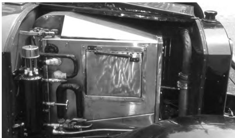
Derr boiler installation in Rolly's 1920 Stanley
