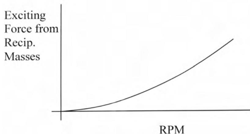
To provide some real numbers, a single-cylinder, single acting, crosshead-type, uniflow expander of 275 cm<sup>3</sup> has the reciprocating mass of 1.7 kg, and 50% of it is balanced. Of 60 mm stroke, the remaining, maximum primary force is then 70 N at 450 rpm, 280 at 900, 1130 at 1800 and 4500 at
